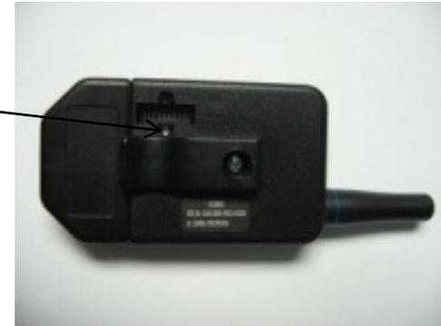
Switches are located on back side of transmitter, on side opposite the antenna, under a small plastic cover. Use the end of a pen to change the position of one or more of the switches.
